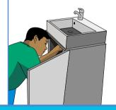
Look out for dripping taps and water stains, mould or peeling material under the sink area. *Did you know a leaking tap can lose up to* 2 *litres of water per hour?*
